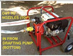
11. Attach the other end of the fire hose from the first pump to the bottom valve of a large pump. You do not need to prime the large pump if a small pump is set up in line before it. Attach another fabric fire hose to the top valve (this hose will be attached to nozzles and/or additional hoses). You may link several hoses end to end in order to lengthen the line. You may use additional pumps in line to maintain/increase water pressure.
