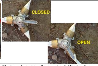
12. If you desire more than one line fighting the fire then attach a 'Y' valve. Multiple 'Y' valves maybe used in sequence to split the line further. A 'Y' valve OPENS all attached hoses if the lever is facing any hose; it CLOSES all attached hoses if it is facing any corner.
