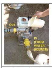
10. If drawing from the ocean or the top of a water tank, you will need to prime the line leading from the water source to the small pump (this is not required if using a fire adapter hose from the bottom of a tank as the water pressure will self-prime the pump). Once both hoses are attached, prime the small pump by removing the black cap and adding water until it overflows.
