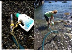
5. In order to avoid the hose sucking debris off the ocean floor tie a float to the end of the hose, or put the end of the hose in a bucket underwater. Man the hose in the water at all times to ensure continuous water flow.
