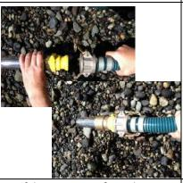
4. If drawing water from the ocean, attach the debris filter to the end of the hard suction hose (green hose). Join multiple suction hoses together for length if necessary.
